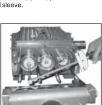
8) Coat the seal sleeve lightly with anti-corrosive grease (e.g. molycote no. Cu-7439) in its fitted area towards the crankcase. Insert the seal sleeves in to their crankcase fittings. Coat the threads of the tension screw (36C) lightly with thread glue and insert it together with a new copper ring (36D) through the ceramic pipe. Turn the pump per hand until the plunger (25) rests against the plunger pipe. Tighten the tension screw at 30 Ft-lbs.
